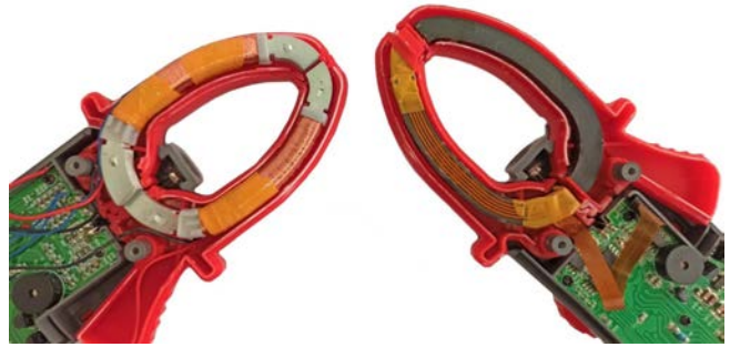
Figura 2. GAF-82C (transformador de corriente CA) vs GAF-82D (Efecto Hall CA/CC)
